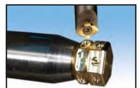
Drilling and milling a groove
