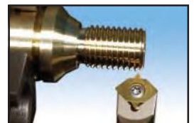
Pitch 0.5-3 mm thread turning external
