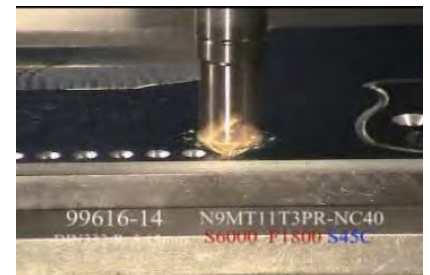
Center drilling by Nine 9 PR insert, spindle speed: 6000 r.p.m. Feed rate: 1800 mm/min. It is 30 times more than HSS center drill.
