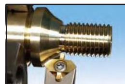
2 mm grooving, depth 4 mm
